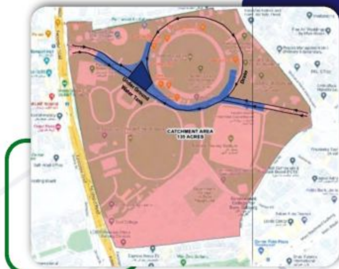
Fig 9: Scheme of Stormwater Storage Tank and drains to eliminate urban flooding at Nishtar Park Stadium Lahore.
