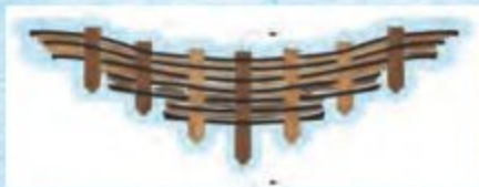
Figure 10 Brushwood Check Dam
