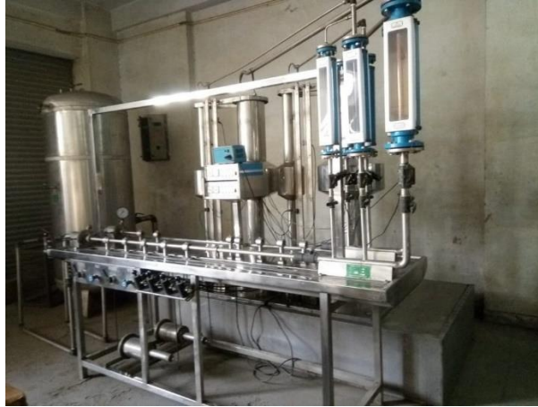
Figure 9-13 Volumetric type test bench
