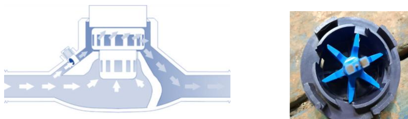
Figure 9-2 Water flow inside a multijet meter and an impeller
