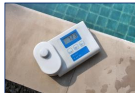
Figure 5-3 Chlorination Test equipment
