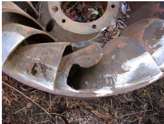
Figure 4-16 Typical cavitation damage of an impeller
