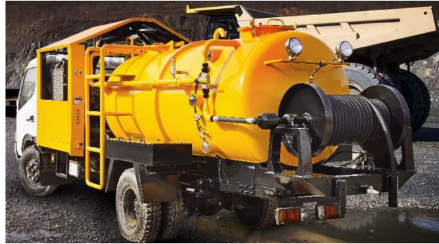
Figure 3-9 Sewer high pressure jetting machine
