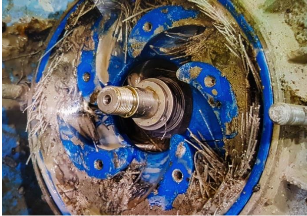
Figure 4-19 Bar screen and a choked impeller
