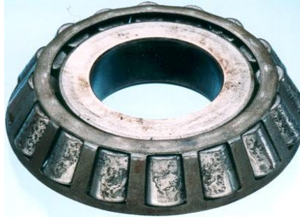
Figure 4-32 Contaminated bearing with water
