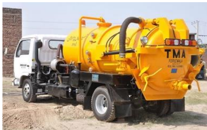
Figure 3-11 Sludge suction machine
